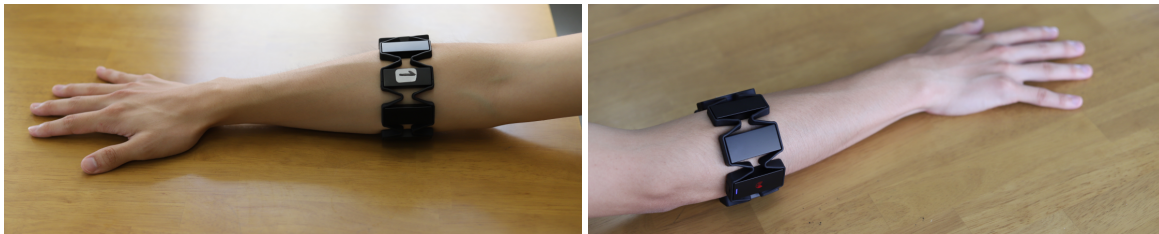
(a) Placement of first sensor: on radio humeral joint about 3cm away from the elbow. (b) Placement of LED light: facing sideways away from the user when the arm is flat on a surface.
